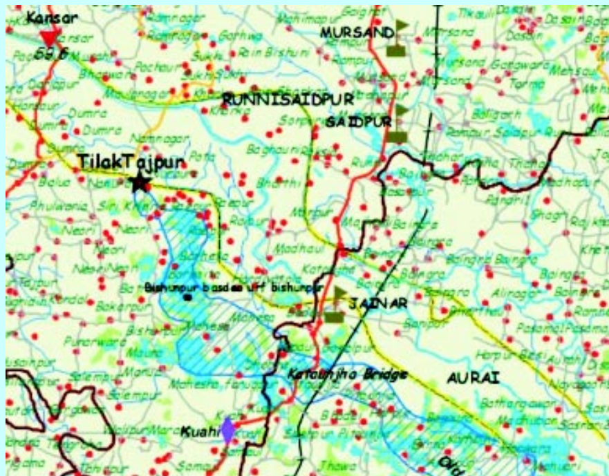
Map 5.9 : Still later we obtained RADARSAT image to map actual extent of flooding. It is notable that the prediction closely matches reality.
